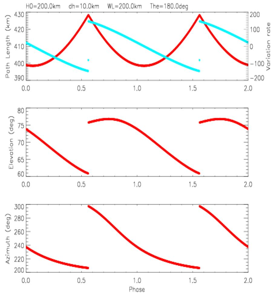
$$\Delta f_{\text{mod}} = \frac{f_0}{C} \frac{dP}{dt} = \frac{f_0}{C} \frac{dP}{d\phi} \frac{1}{T}$$
