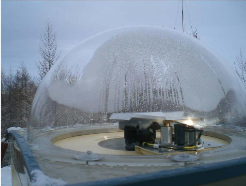
**Camera: condensation inside the dome after rain/snow.**
