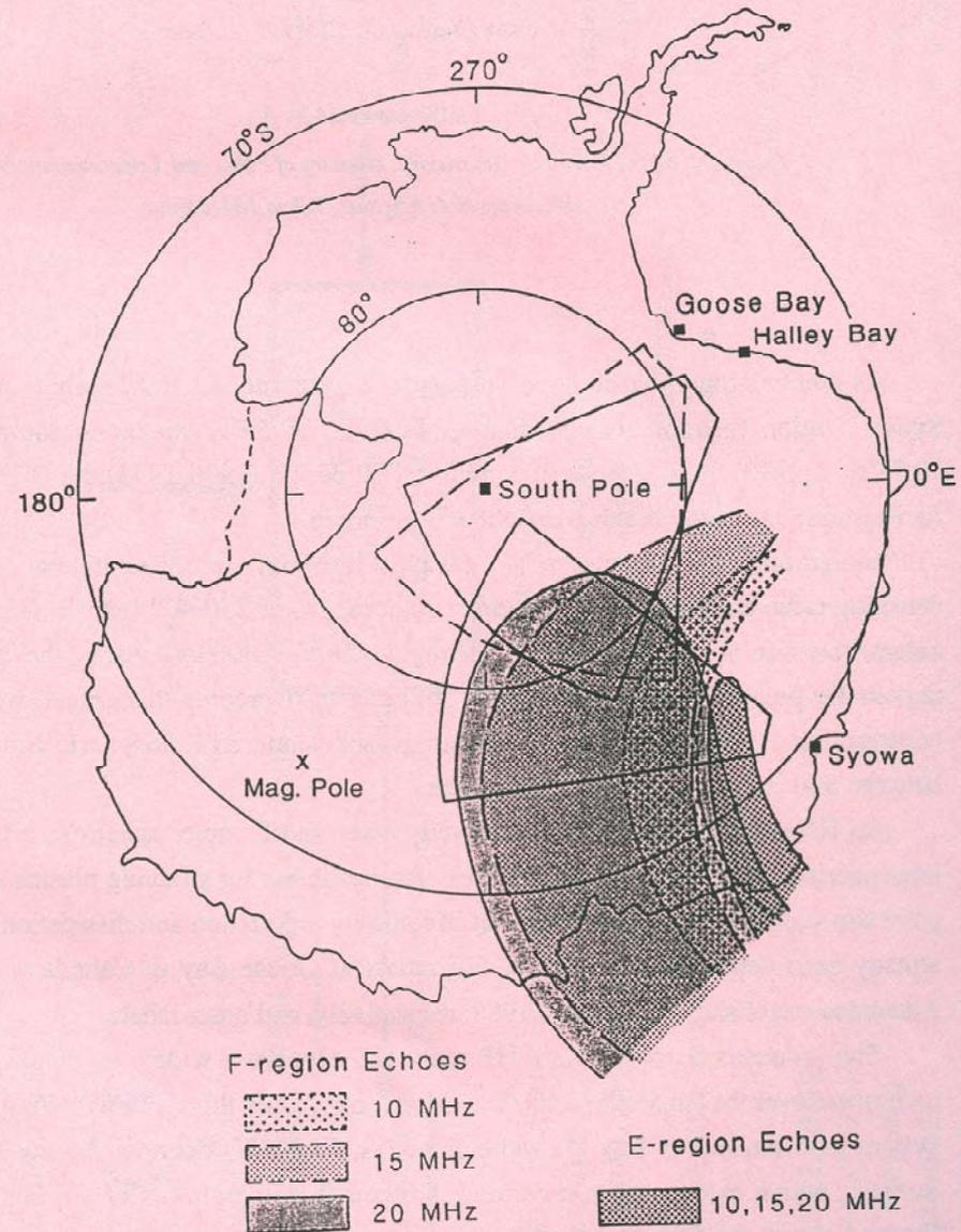
Fig. 2. Schematic illustration of viewing areas by Antarctic twin HF radars (B) and Canadian twin HF radars (A). A and B make a geomagnetically conjugate pair.
