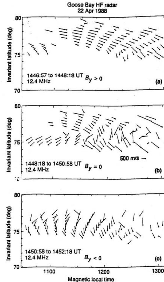
Fig. 7. Goose Bay radar observations of the temporal variation of F-region plasma drift patterns in the vicinity of the cusp and cleft as IMF  $B_y$  changes from positive to negative and  $B_z$  remains negative (From Greenwald *et al.*, 1990).
