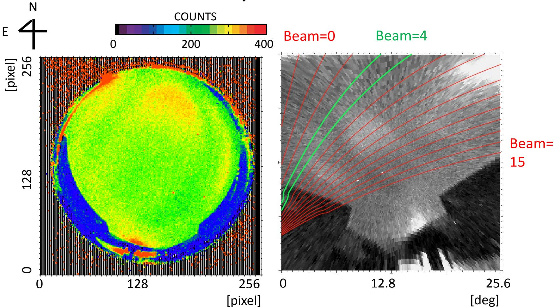
(left) An example of 630-nm all-sky airglow image. (right) The projection of the image onto the geographical coordinates. The red and green lines indicate beams of the HF radar in the field of view (16<sup>th</sup> Jan. 2010 1602UT).
