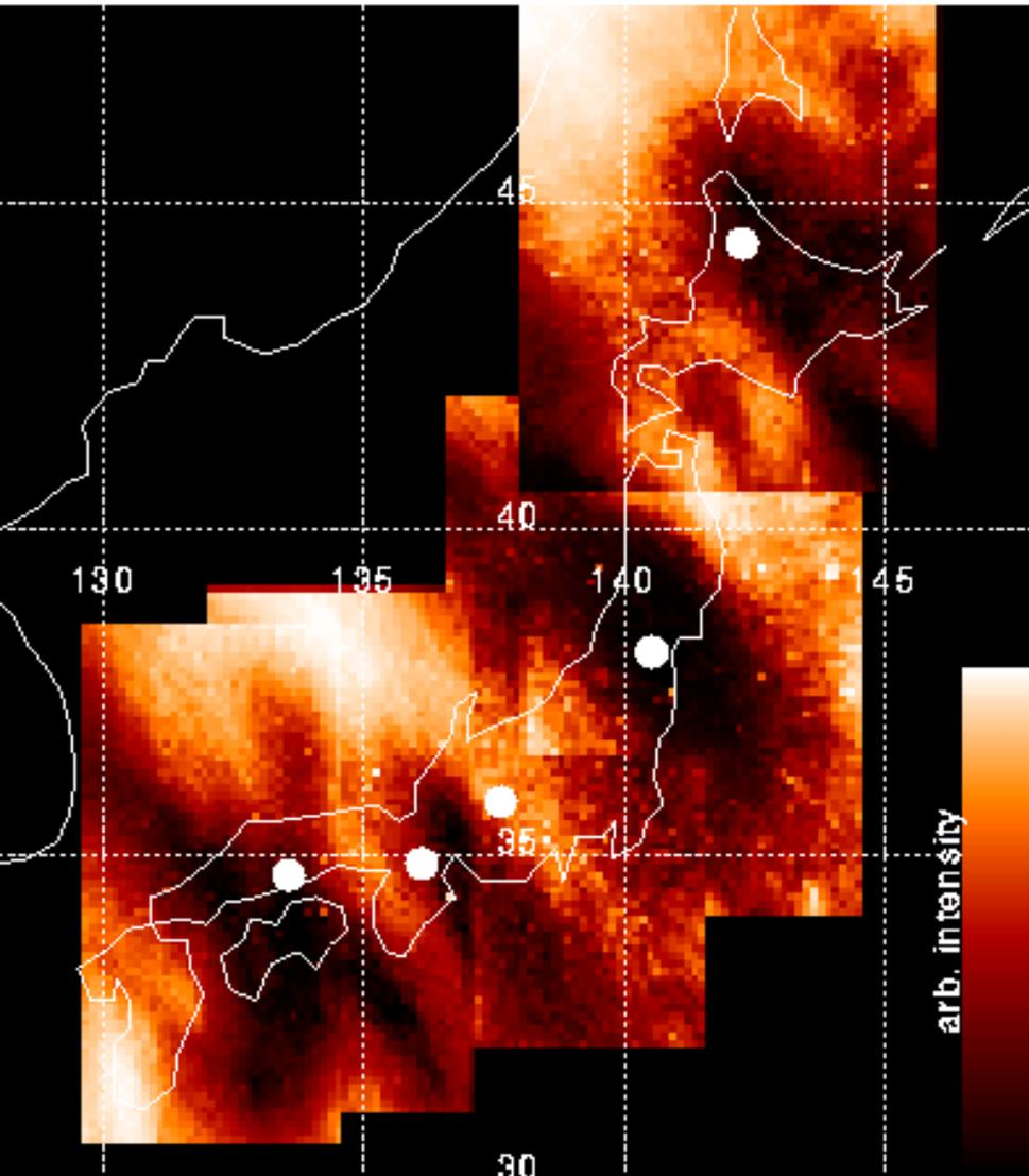
MSTID is a kind of ionospheric disturbances with a horizontal scale of 150-500 km.
