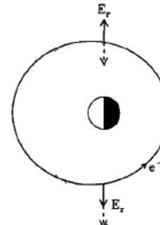
**Figure 2.** Sketch of an electron drift path in a compressed dipole, with electric fields indicated for an  $m=2$  mode. Solid arrows indicate the electric field at  $t=0$  for an electron starting at dusk, while the dashed arrows indicate the electric field direction half a drift period later.
