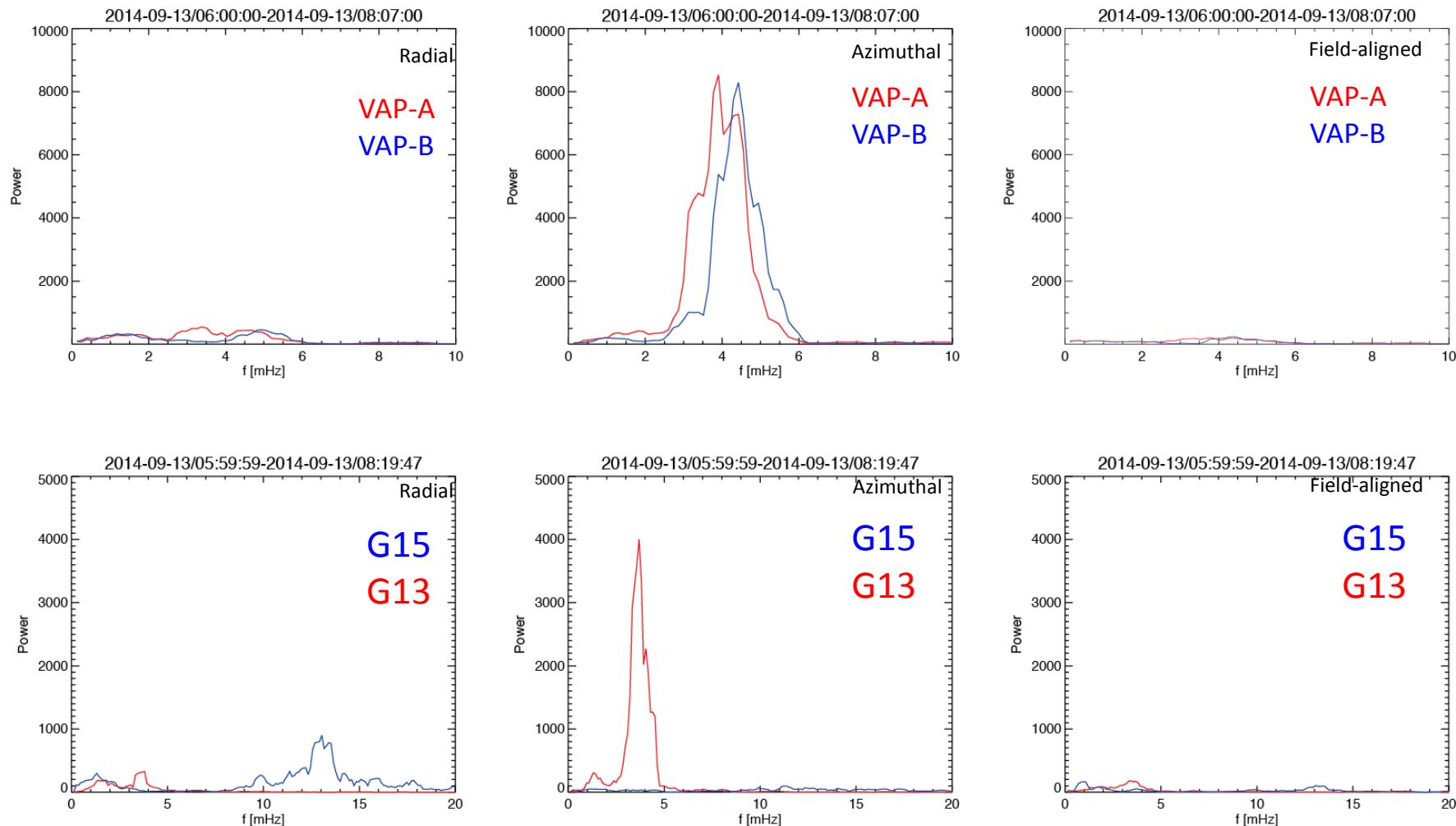
toroidal mode with 3.8 mHz (VAP-A and GOES 13)
