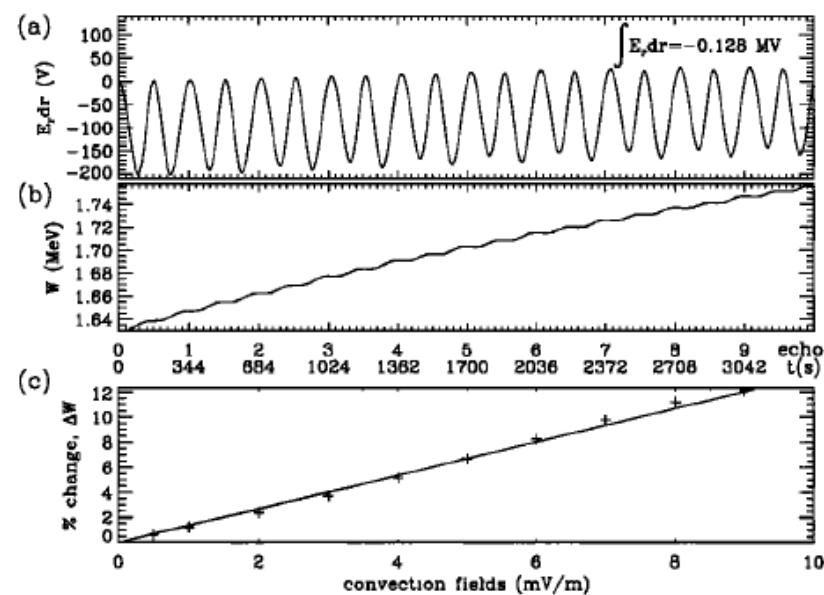
**Figure 3.**  $E_{r,dr}$  (a) and energy (b) as a function of time and drift echoes for an electron with initial energy of 1.63 MeV, moving in a 3 mHz,  $m=2$  toroidal field of amplitude 3 mV/m. (c) Relative increase in energization for same particle, as a function of increasing dawn-dusk convection electric field.
