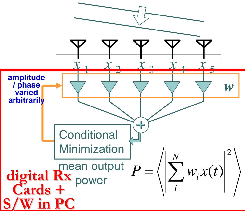
Each antenna output separately record through digital Rx, any Rx beam-forming in SW in PC
