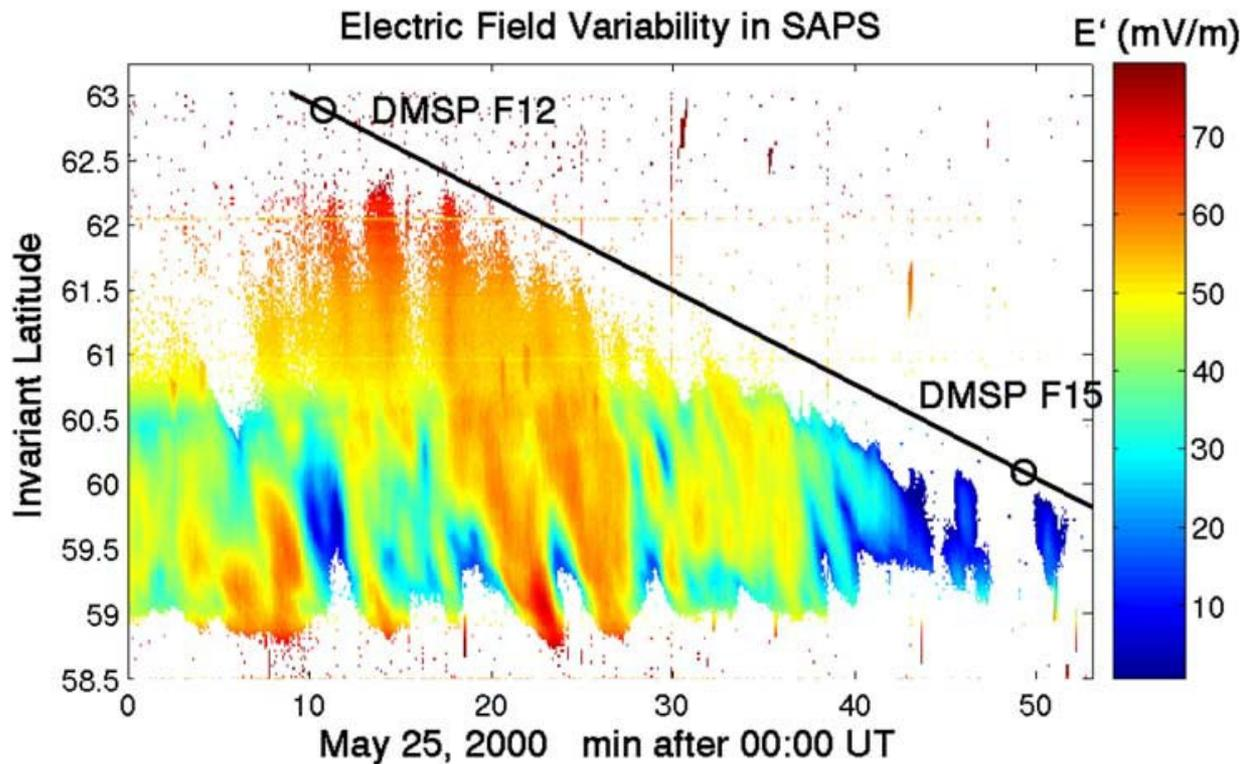
In fact, the color-coded values in the left panel are **not electric field vector component**, but electric field **variability** based on the strength of backscatter echoes due to 2-stream instability.
