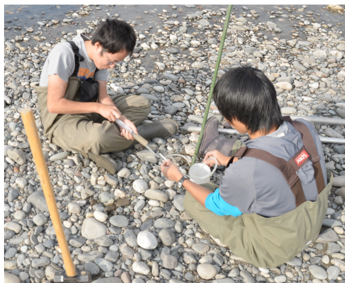
Figure 2 Method for sampling hyporheic water for testing water quality. (a) Penetration of standpipe for installation of water suction tube. (b) Collection of sample water by sucking up using a cylinder of 100cc in inner volume.
