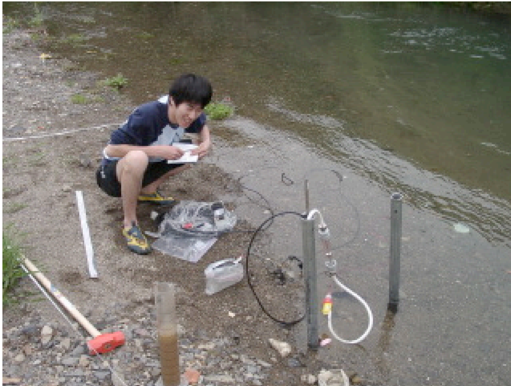
Figure 3 Measurement of hydraulic conductivity by the Packer Method in the field. Constant water flow is installed by an electric pump measuring the water level in the standpipe.
